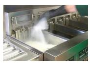
Miracle Filter Powder can be simply cast into the oil or spread evenly over the filter paper
